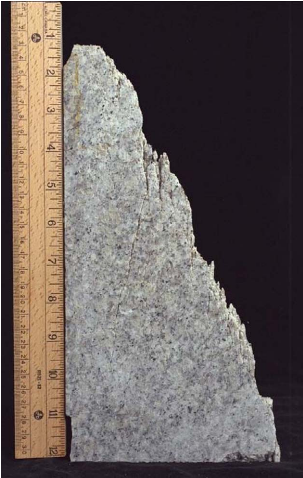
Fig. 2. Photograph of a failed sample, illustrating both axial cracking and macroscopic shear plane.
